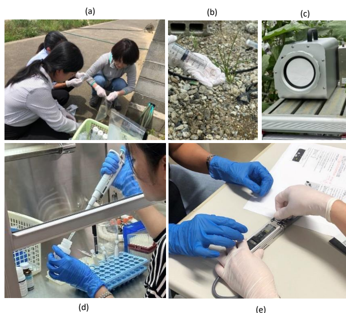
Figure 27. Water filtration during sampling (a, b); Bioaerosol sampling (c); DNA extraction (d); Nanopore sequencing (e)
